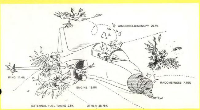
Figure 2 Impact Point on Aircraft
